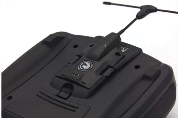
JR bay with installed TBS Crossfire module
