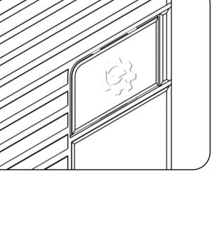
Short press the right button to switch and check voltage of each cell. (Voltage accuracy for each cell: within ±0.05V from the actual voltage generally.)
