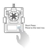
Note: When the RFTX module is entering menus page, the binding between RFTX module and receiver will be lost, the binding will recover after exiting menus page automatically; you must re-power the receiver if you have changed the Pkt Rate.
